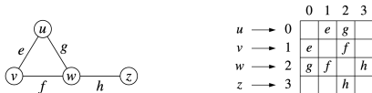
Figure 7: Left: An undirected graph G ; Right: a schematic representation of the auxiliary adjacency matrix structure for G , in which n vertices are mapped to indices 0 to n-1 .
